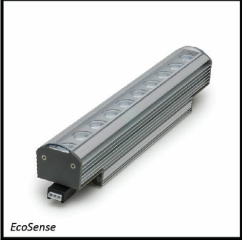
Figure 3.06 Surface-mounted linear luminaires for a cove or slot. A typical asymmetric beam angle for a wall-grazer is a15 x b60 degrees.
