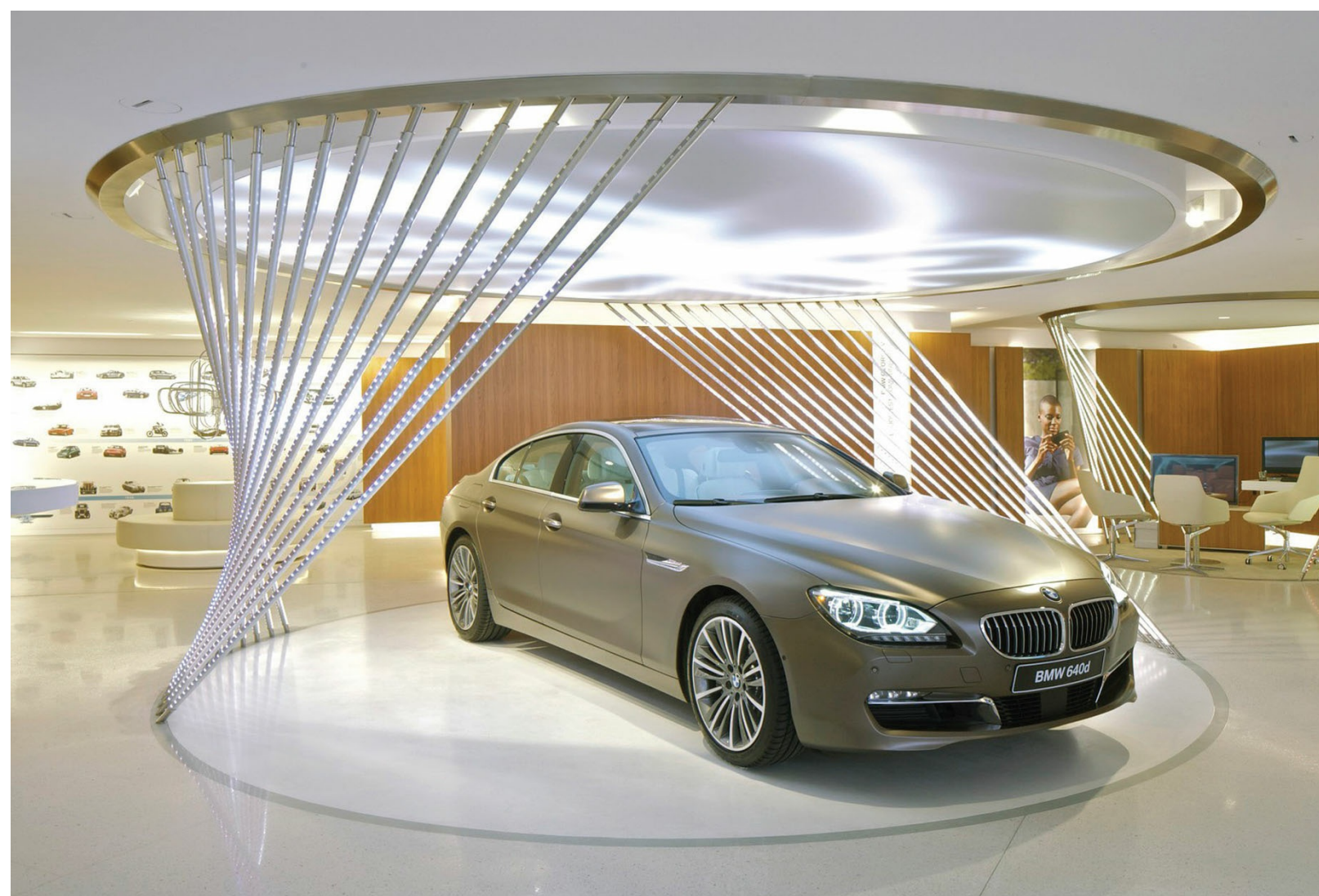
Figure 6.67 Light panel over the BMW create swage line on the car. Spot light are hidden in the slot. (Arch: Carbondale; Lighting: Mindseye; Photo: Andy Spain)
