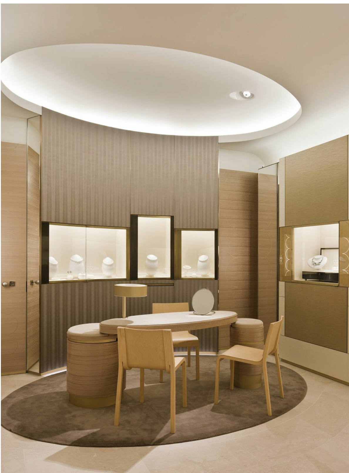
Figure 6.25 A well-lit coffer using tiltable linear LED – standard 120 degrees.
