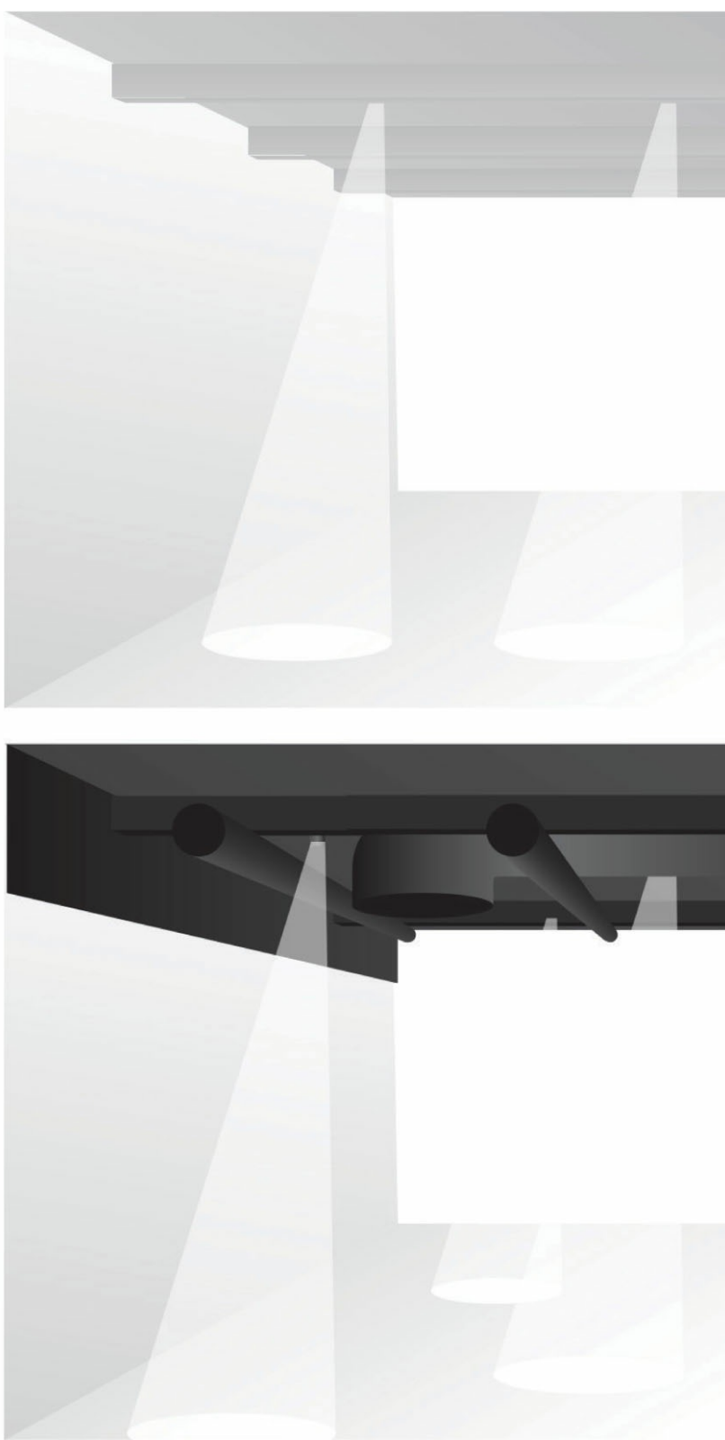
Figure 3.21 Light hidden. (Above) a white finished ceiling with exposed beams. (Below) a busy ceiling with all services exposed painted in black.
