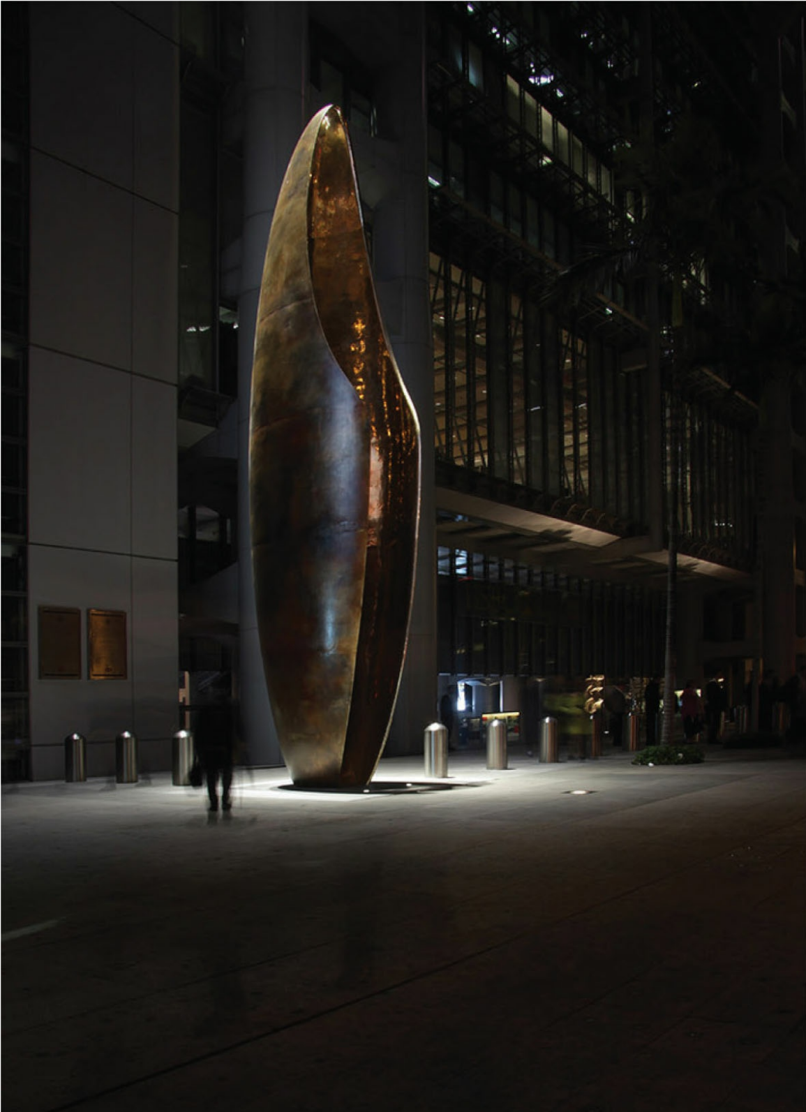
Figure 4.38 Main light provided by two lights from above, grounding the statue. Three floor recessed uplights are highlighting the nose and the wings of the Grain of Rice sculpture from BASED UPON, for HSBC Hong Kong.
