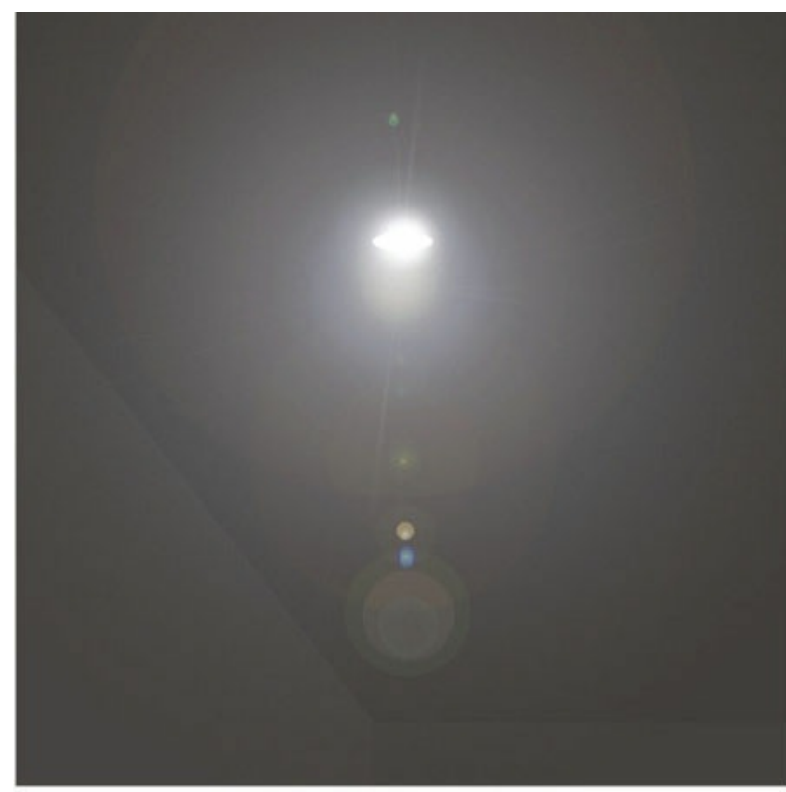
Figure 4.41 Left: glare caused by strong directional point light in a dark ambient. Right: diffused panel light creating a lighter ambient causing no glare.
