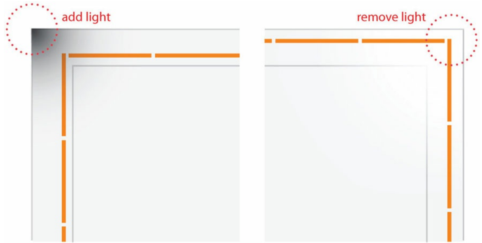
Figure 6.27 Topview of lighting in a ceiling coffer.
