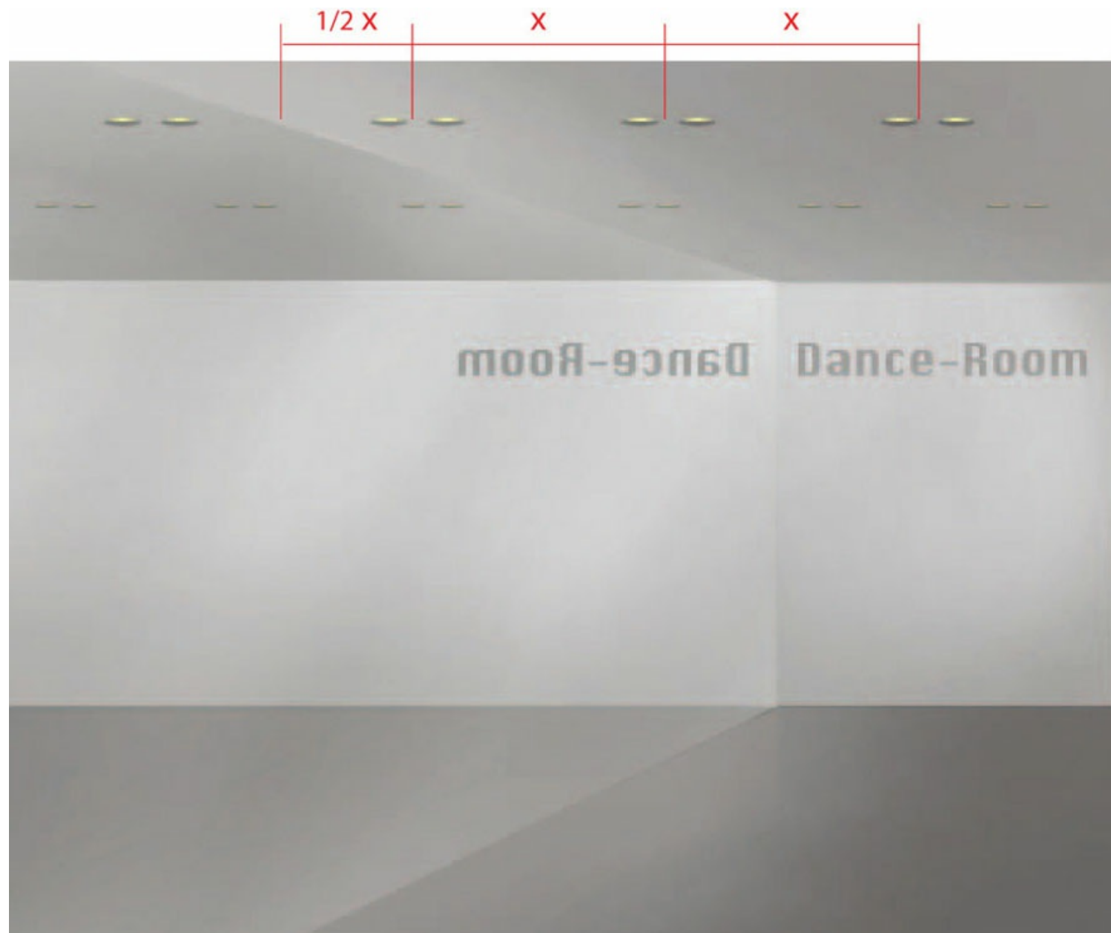
Figure 6.44 Mirror lighting continues seamless into the mirror.
