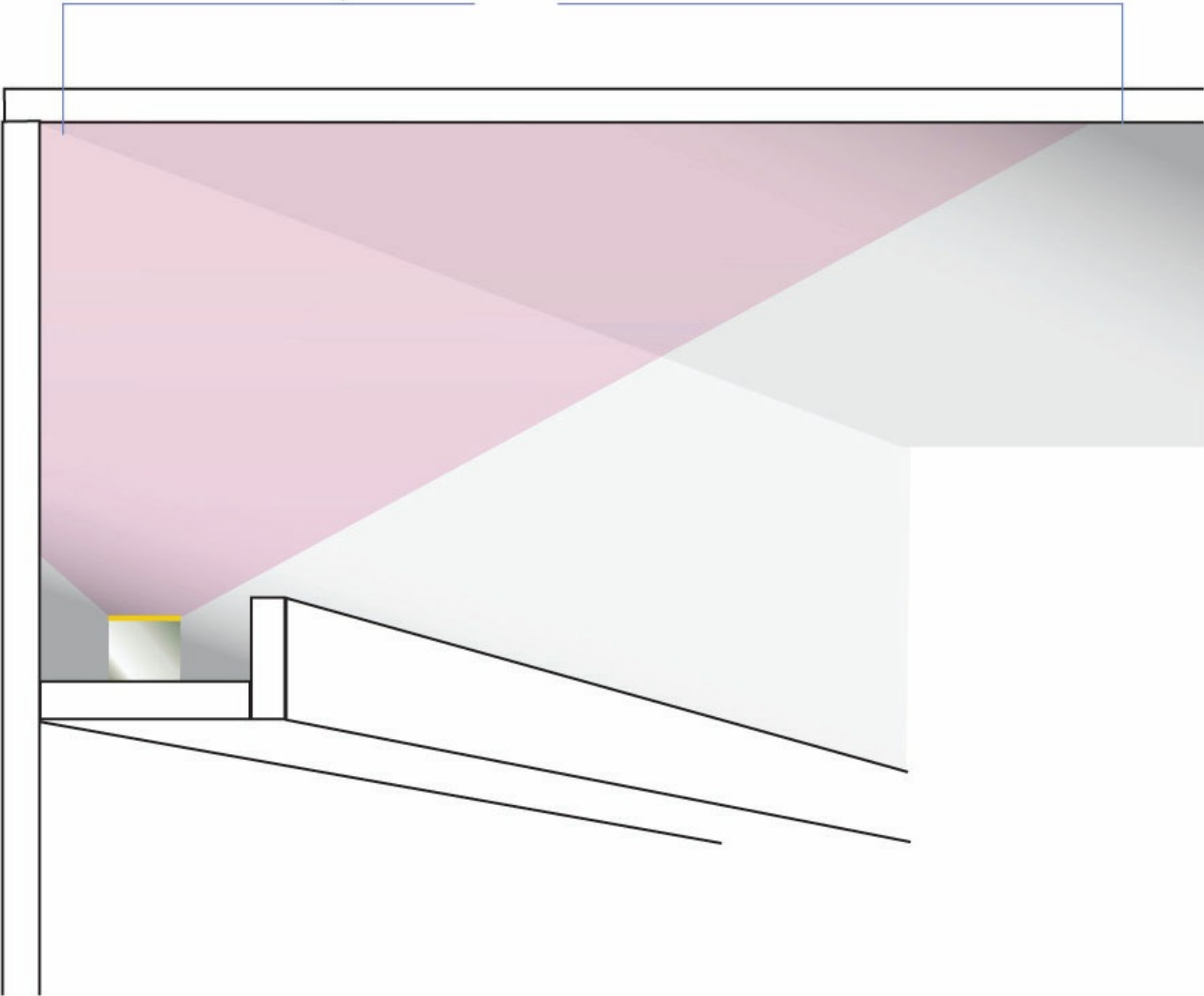
Figure 6.23 A good distance of the cove to the wall, but the defined beam angle of the luminaire creates a shadow on the ceiling.
