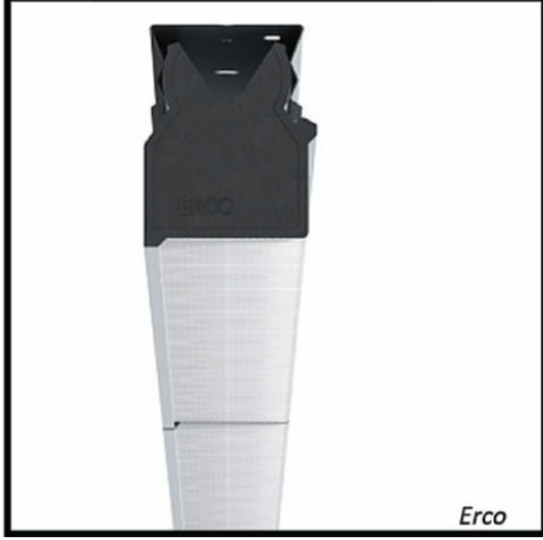
Figure 3.06 Surface-mounted linear luminaires for a cove or slot. A typical asymmetric beam angle for a wall-grazer is a15 x b60 degrees.
