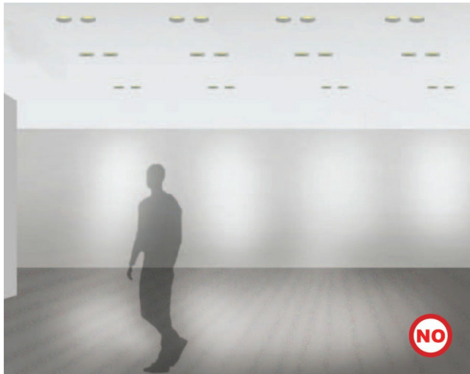
Figure 6.50 Top-heavy - single luminaire usage.
