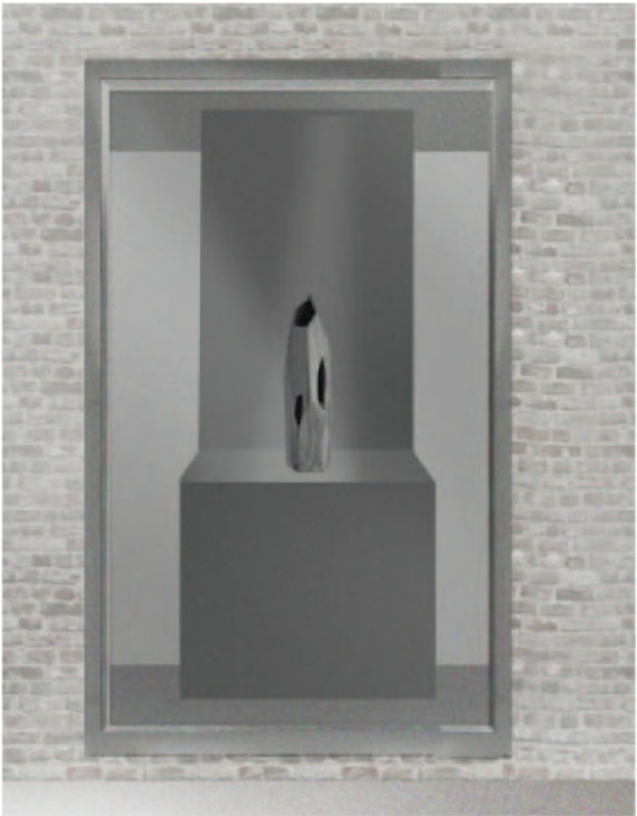
Figure 6.39 Shopwindow lighting not able to compete with bright exterior sunlight.
